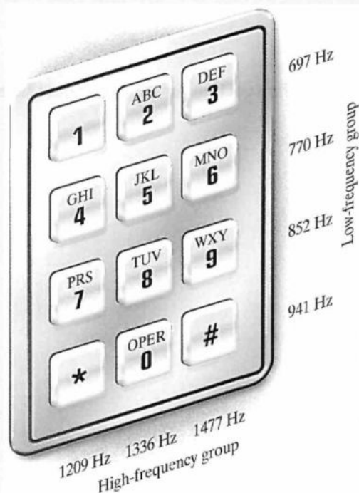
Figure 14.32 ▲ Tones generated by the rows and columns of telephone pushbuttons.
