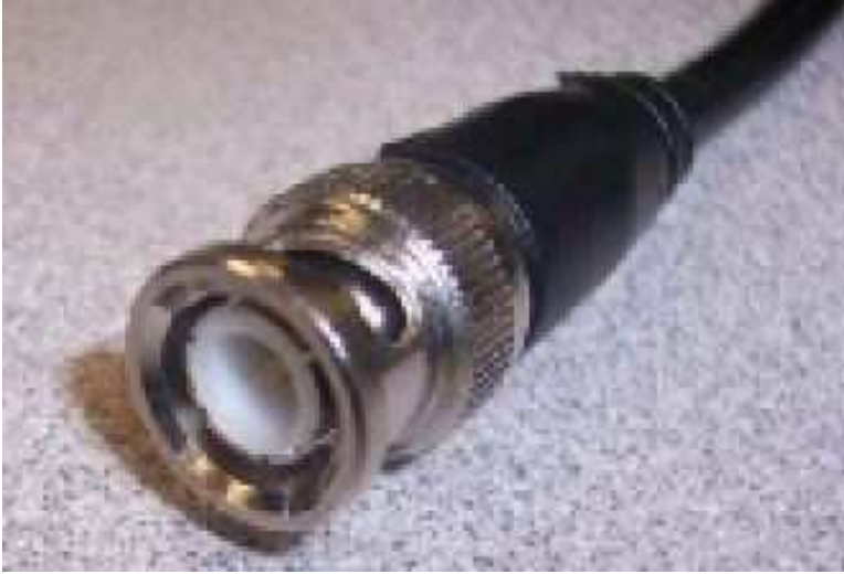
Figure 11.9: A BNC connector on a coaxial cable
