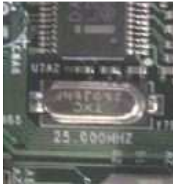
Figure 9.5: A crystal oscillator on a circuit board
