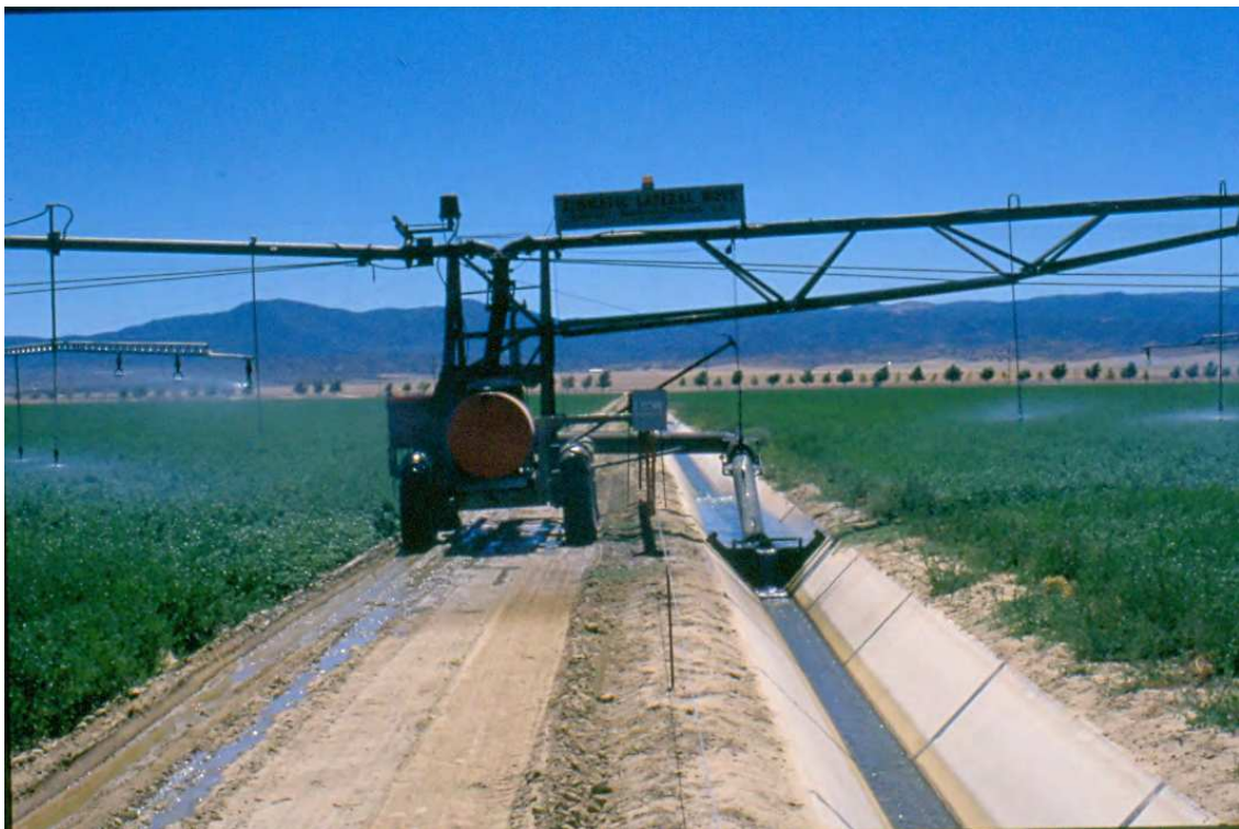
Plate 52 Feeder system for modern linear move
