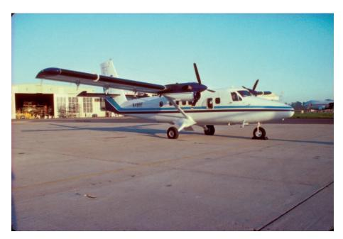
Figure 4 NOAA Twin Otter survey aircraft with bubble window (under propeller) and belly window port (above tire) (Photo: K. Forney).
