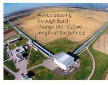
wave detectors consist of two long tunnels at right angles
