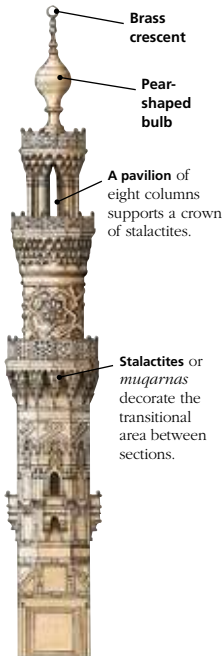
This three-tiered spire, adorning the Mosque of Qaitbey (see p102), displays the elaborate decorative stonework typical of late Mamluk minarets.
