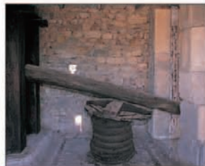
Reconstruction of an oil press, showing the baskets used for pressing the olives
