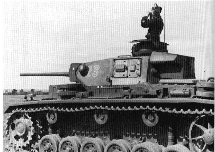
Plate 203. Pz Kpfw III Ausf J or L; note that the gunner's vision port on the side of the turret has been eliminated.
