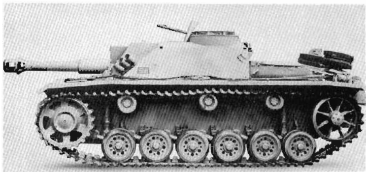
Plates 261-262. StuH42 based on the StuG III Ausf F (top) and the Ausf G (below).
