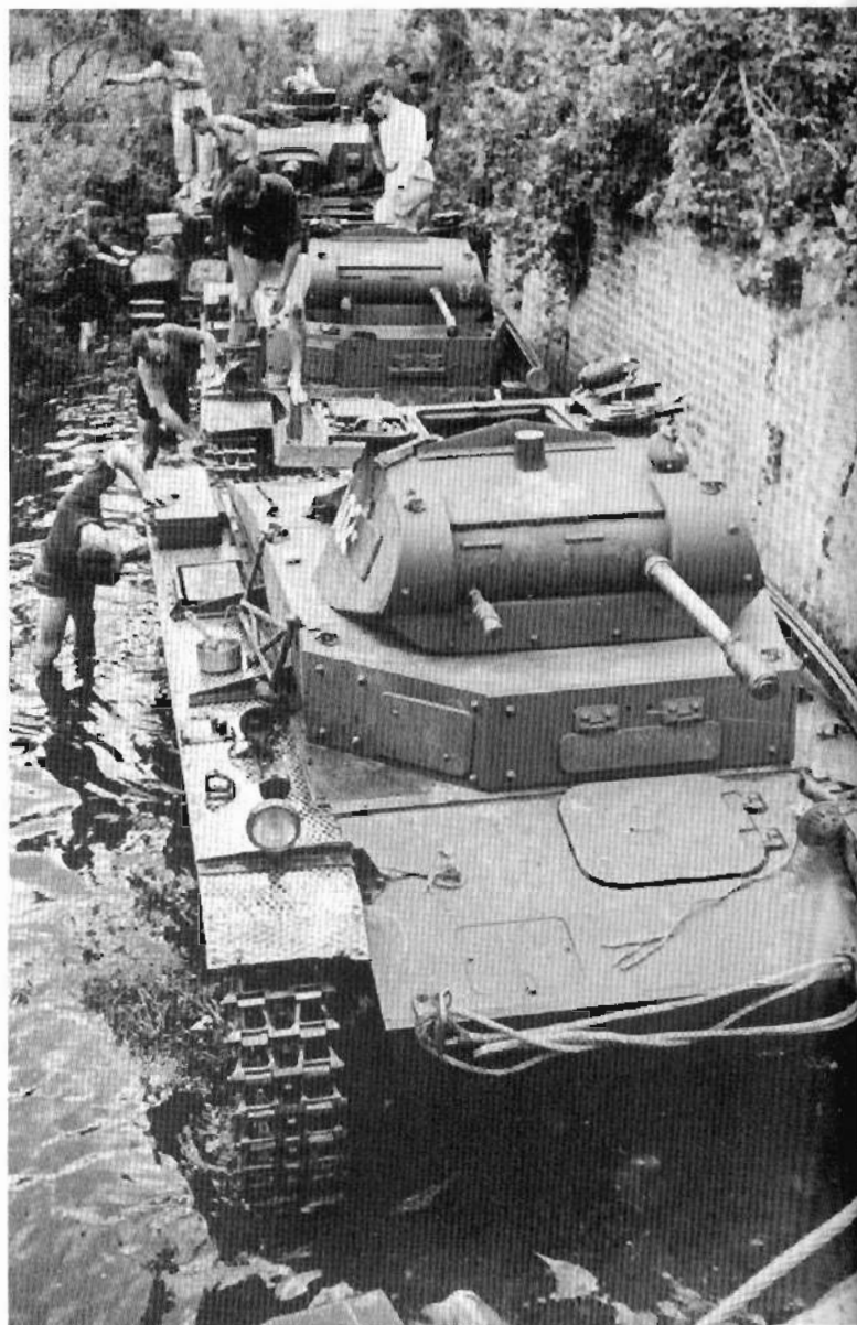
Plates 76-77. A comparison of hull fronts: the top photograph shows the rounded shape of the early models, Ausf c, A, B and C, while the lower view shows the Ausf c, with additional armour plate bolted to the hull front. The second vehicle in this lower photograph is an Ausf A, with different driver's visor and vision ports.
