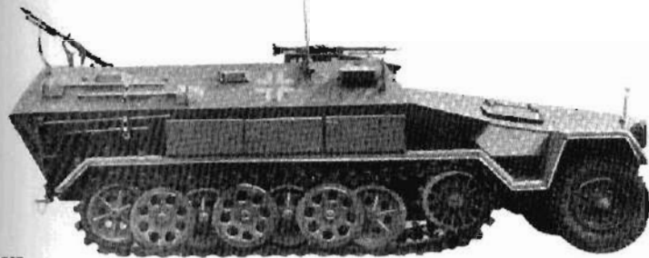
Plates 587-590. Sd Kfz 251 mittlerer Schützenpanzerwagen Ausf A (Plate 587), Ausf B (Plate 588) and Ausf C (Plates 589 and 590). Note that the vehicle in Plate 590 has a riveted body.
