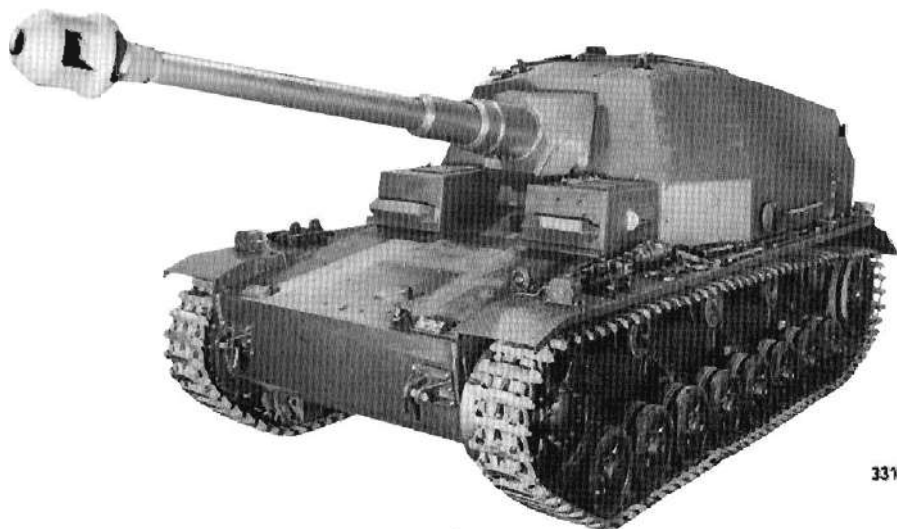
Plates 330-332. 10.5cm K18 auf Pz Sfl IVa. Plate 330 shows the vehicle on operations in Russia.
