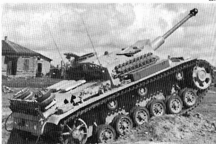
Plates 257-259. StuG III Ausf G. (Note, in Plate 259, the additional armour bolted to the front of the vehicle.) Plate 260 (opposite page, top). StuG III Ausf G with Saukopf gun mantlet.
