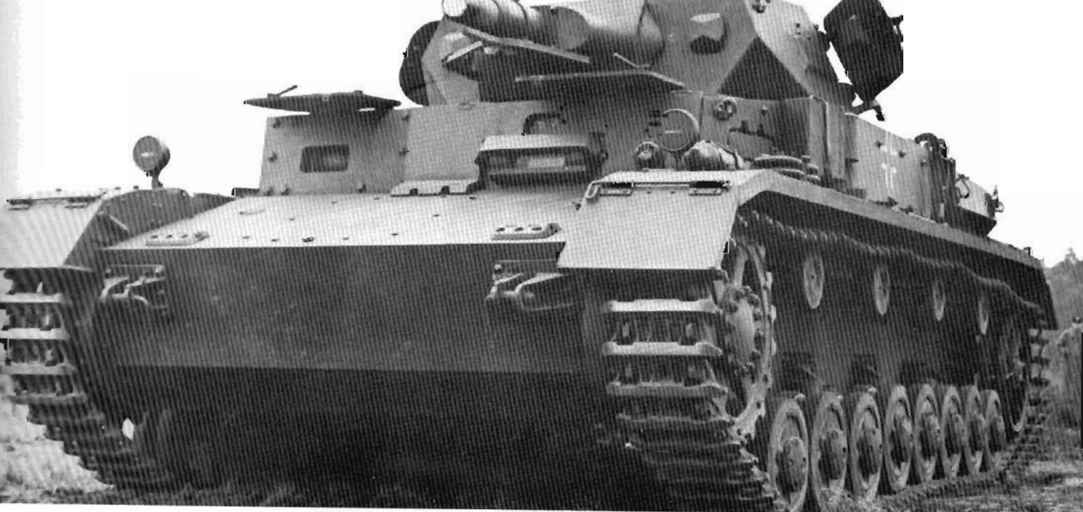
Plates 293-295: Pz Kpfw IV Ausf E. Above right, a factory photograph that shows the new driving sprocket, new driver's visor (Fahrersehklappe 30) and the extractor fan in the turret roof; below, in North Africa.
