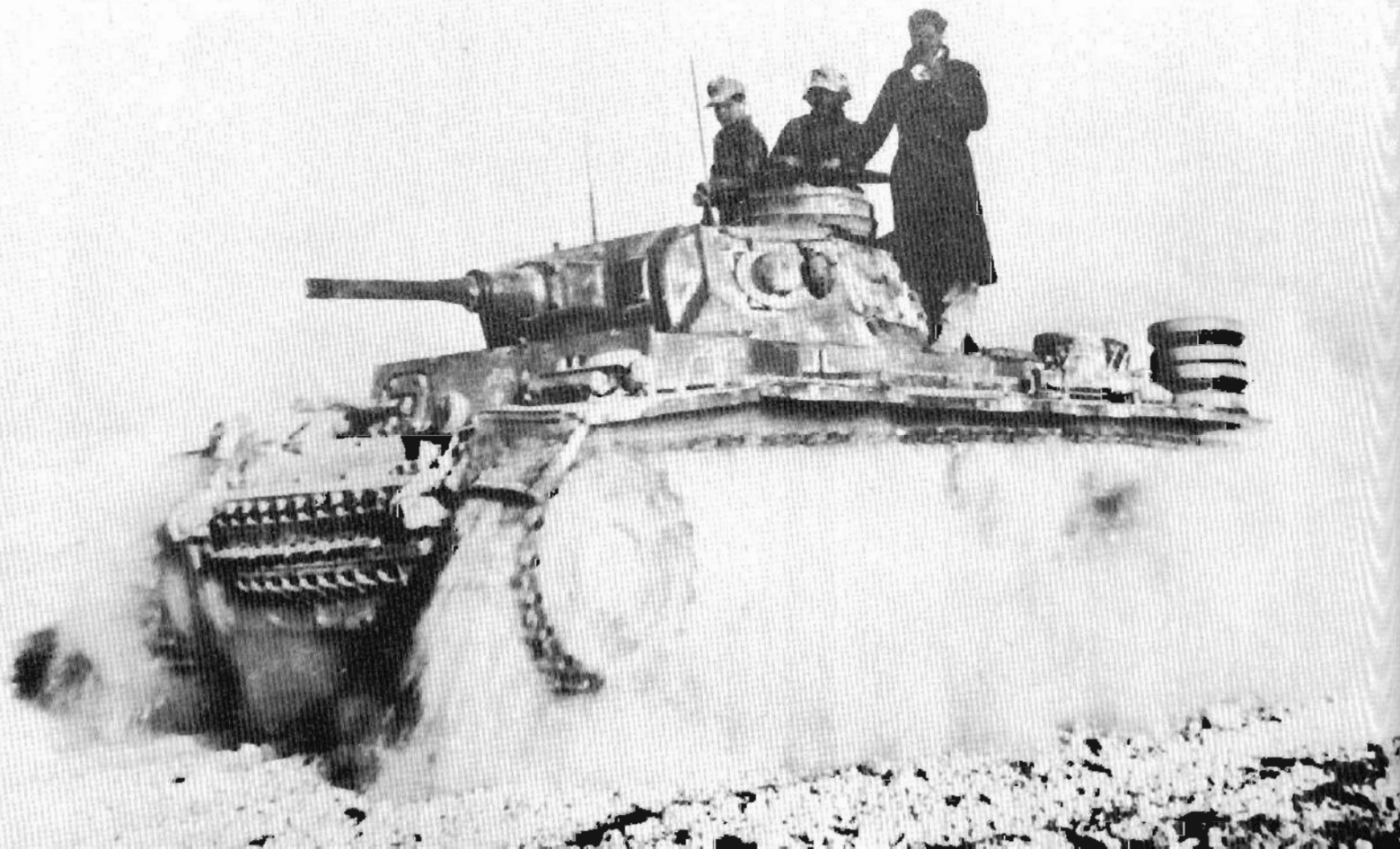
Plates 195-198. Pz Kpfw III Ausf H. A new type of drive sprocket, with six D-shaped holes and open eight-spoked rear idler, was introduced with this model. Note the 30mm armour plates bolted on to the upper and lower nose plates. Above, in Sofia, 1941; below, at speed in North Africa.
