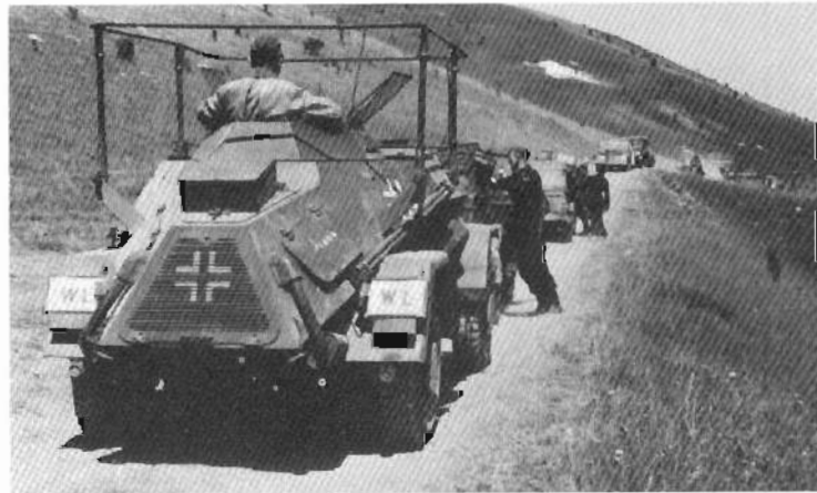
Plates 712-714. Le Pz Sp Wg (Fu) Sd Kfz 223. Note that the frame aerial is raised in Plate 714, lowered in Plate 712.
