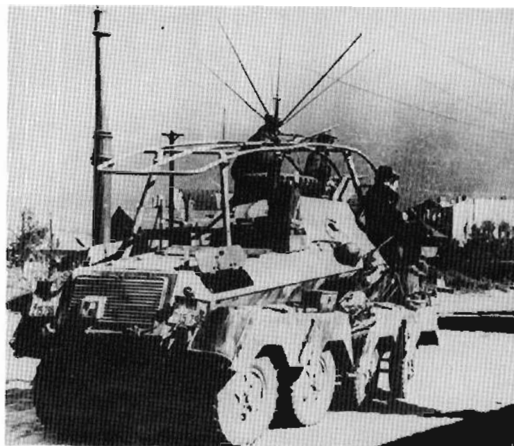
Plates 740-742. Pz Fu Wg (Sd Kfz 263) 8-Rad, showing the star aerial open (Plate 740), the mast telescoped down (Plate 741) and the MG34 (Plate 742).
