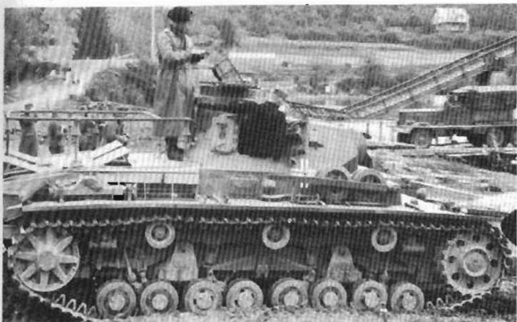
Plates 219-220. Pz Bef Wg III Ausf D 1 , showing the large frame antenna and the dummy 3.7cm gun.
