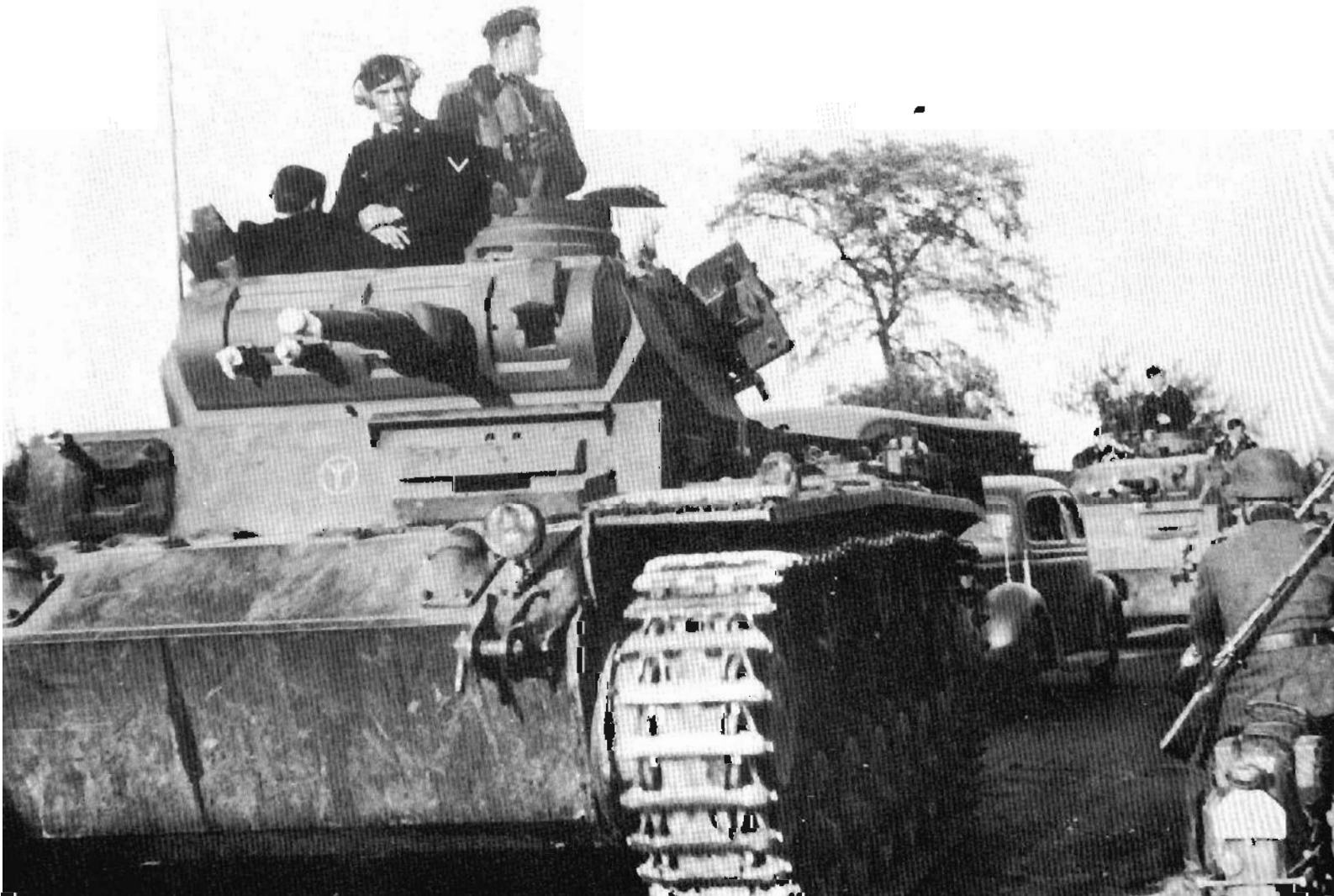
Plates 190-191. Pz KpW III Ausf F. The vehicle shown above carries the 5cm KwK L/42 gun in an external mantlet.
