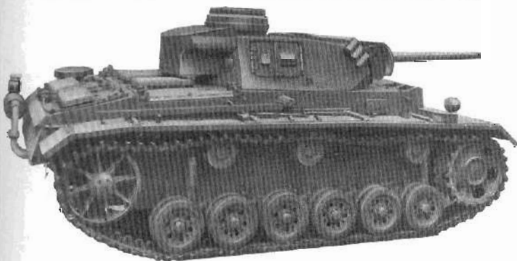
Plates 206-207. Pz Kpfw III Ausf M. Note the modified exhaust valve for deep wading and the absence of both the hull escape hatch and the loader's vision port in the turret side. Right: vehicles equipped with Schürzen (apron armour) on the Russian Front.
