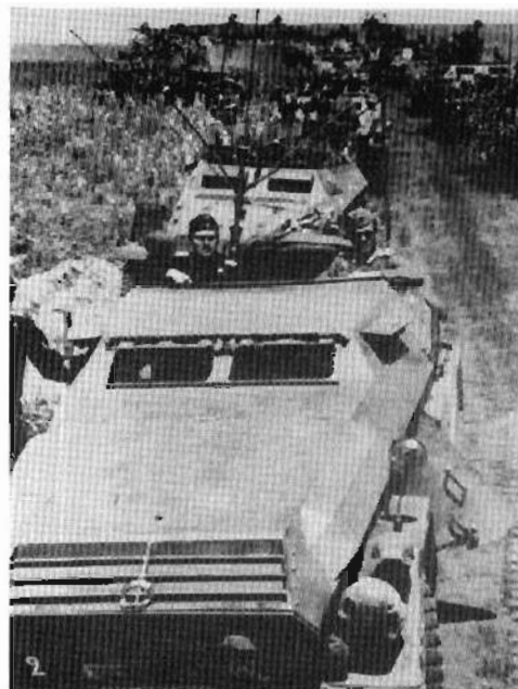
Plates 757-758. S gl gep PKW (Sd Kfz 247) Ausf A. Plates 759-760. S gl gep PKW (Sd Kfz 247) Ausf B, based on the 4 x 4 chassis with frontal armour shield and star aerial (Plate 760).
