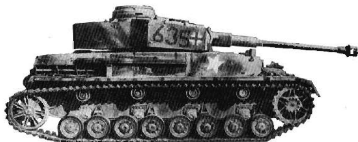
Plates 305-307. Pz Kpfw IV Ausf H. The vehicle in Plate 305 has the new type of drive sprocket but the old type of idler wheel; Plate 306 shows a late production model, with both new drive sprocket and idler wheel. Plate 307 (below): on manoeuvres in France in 1944.
