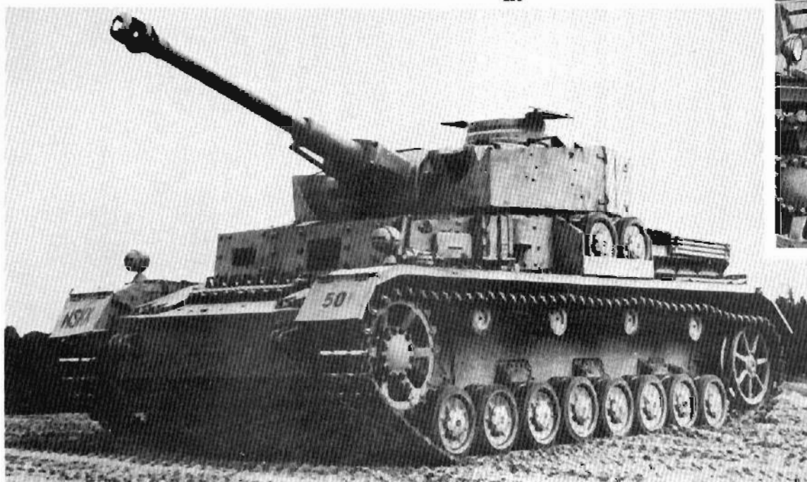
Plate 289. Pz Kpfw IV Ausf D, in service at a tank driver school, exhibiting the later types of cupola and drive sprocket. (The machines in the background are Fahrschulwanne IV tank training vehicles.)
