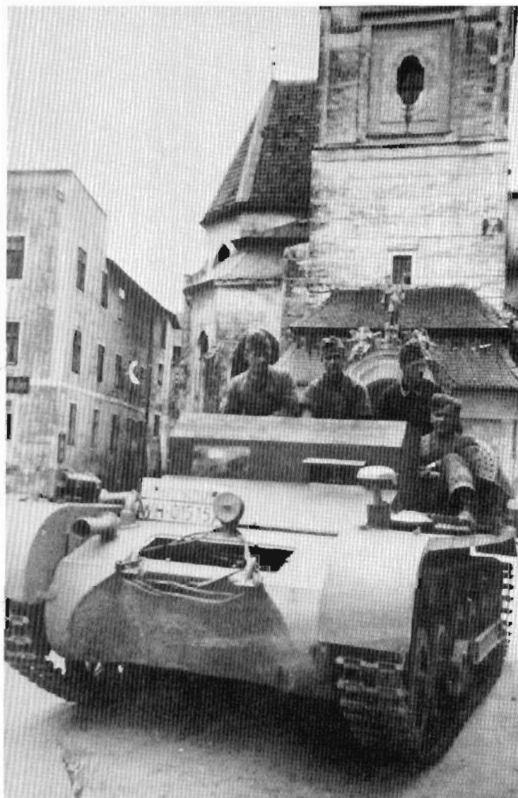
Plates 47-48. The modified driving school vehicle based on the Pz Kpfw I Ausf B and driven by gas.
