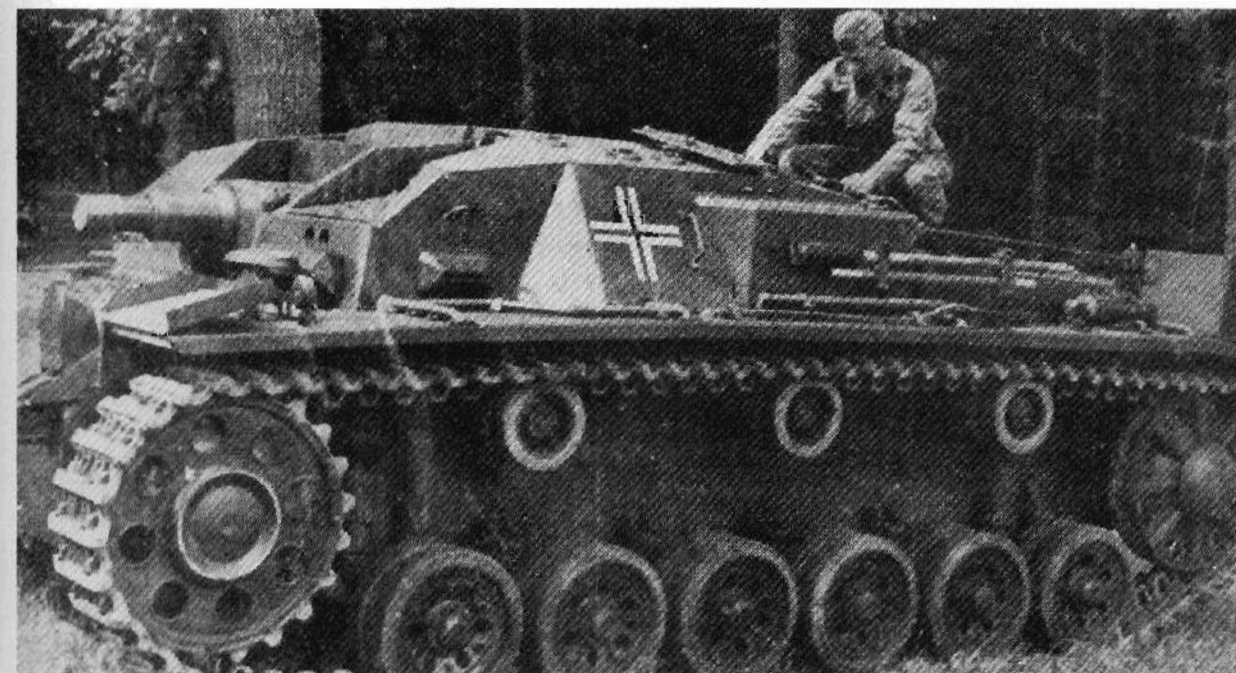
Plates 244-245. StuG III Ausf A (showing the Pz Kpfw III Ausf F suspension). Plate 248. One of the prototype (0-series) vehicles.
