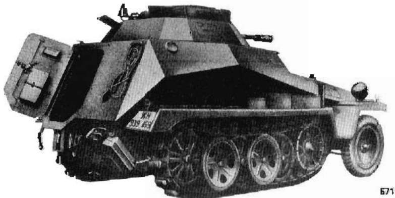
Plates 571-574. Sd Kfz 250/9 leichter Schützenpanzerwagen (2cm). That in Plate 573 is based on the 'Neu' vehicle, as well as having the later Hängelafette (see page 192). Below, vehicles operating in Russia.
