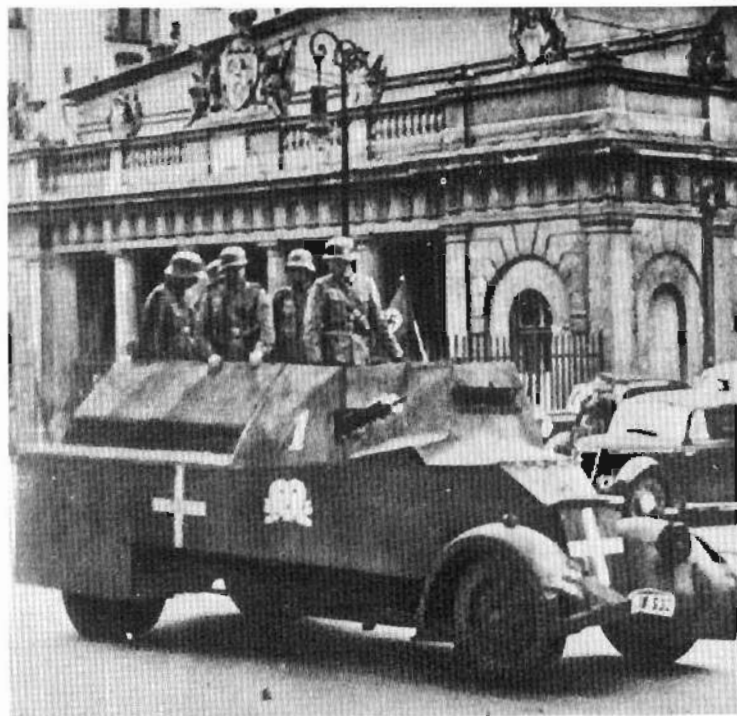
Plates 761-763. Police armoured cars: ADGZ (Plates 761-762), and a Strassenpanzerwagen (Plate 763). The latter was one of a number of commercial vehicles armoured for use by SS police patrols and armed with the Maxim MG08 machine-gun.
