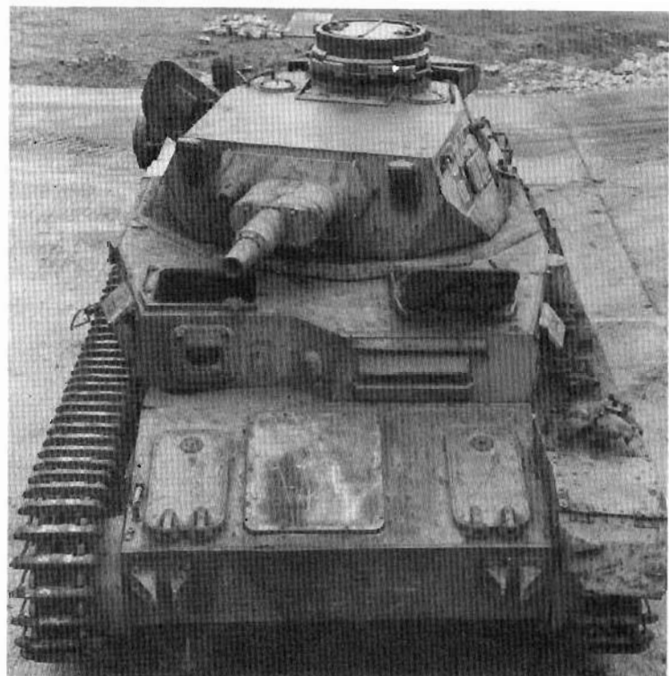
Plate 285. Pz Kpfw IV Ausf D. Note that the hull machine-gun position has been re-introduced within the Kugelblende 30.
