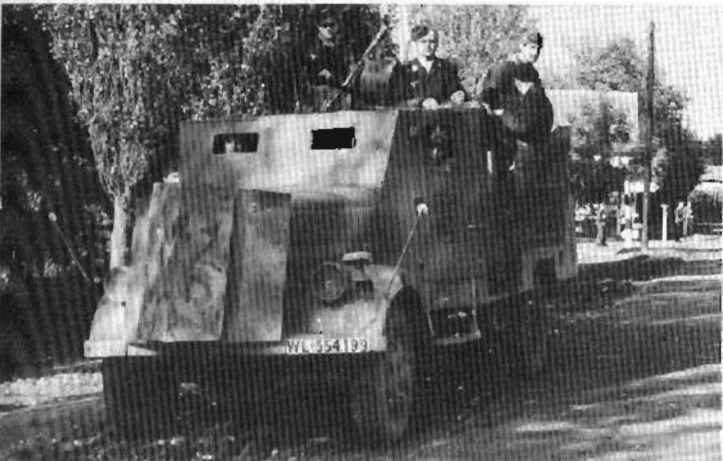
Plate 767. 2cm FlaK38(Sf) auf LKW (Opel Blitz)—a converted medium truck, with armoured front and drop sides. Plate 788. 2cm FlaK30(Sf) auf s gl Einh PKW. Plate 769. 2cm FlaK38(Sf) mounted in the standard passenger body.
