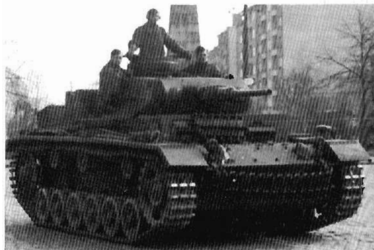
Plates 195-198. Pz Kpfw III Ausf H. A new type of drive sprocket, with six D-shaped holes and open eight-spoked rear idler, was introduced with this model. Note the 30mm armour plates bolted on to the upper and lower nose plates. Above, in Sofia, 1941; below, at speed in North Africa.
