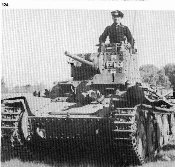
Plates 124-125. Pz Kpfw 38(t) Ausf A. The lower photograph shows the curve of the driver's plate and the hull-mounted machine gun.
