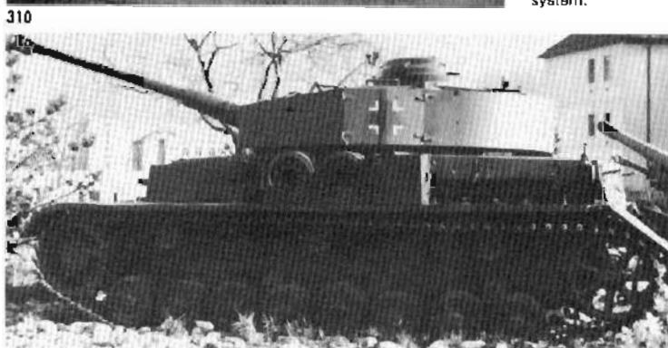
Plates 308-312. Pz Kpfw IV Ausf J: Plate 308, with Schürzen; Plate 309, with wire mesh side-skirts; Plate 310, a top view showing the turret after elimination of the vision ports and loader's vision port in the turret front; Plate 311, with three track-return rollers; Plate 312, a rear view showing the new exhaust system.
