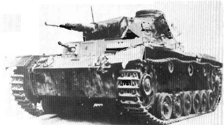
Plates 190-191. Pz KpW III Ausf F. The vehicle shown above carries the 5cm KwK L/42 gun in an external mantlet.
