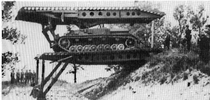
Plates 365-367. Brückenleger IV. Top, the Krupp version positioning its bridge. Plates 366-367, the Magirus version, left, launching its bridge.
