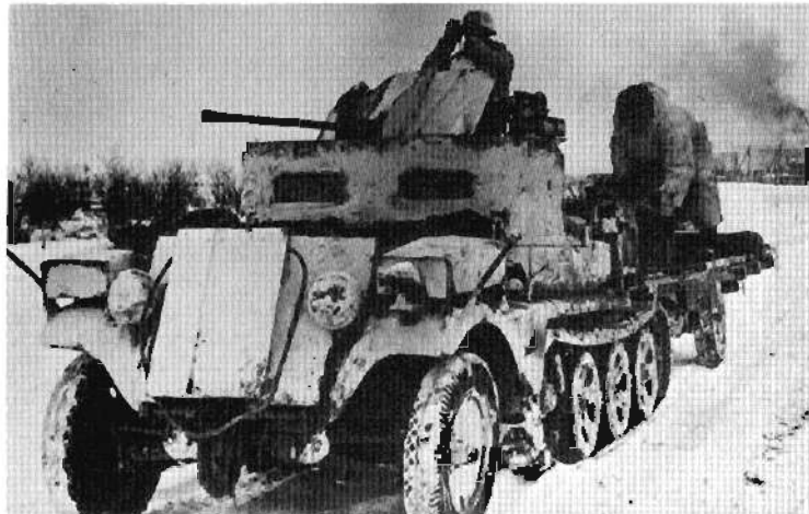
Plates 657-668. Sd Kfz 10/5; right, with armoured cab and 2cm FlaK38.
