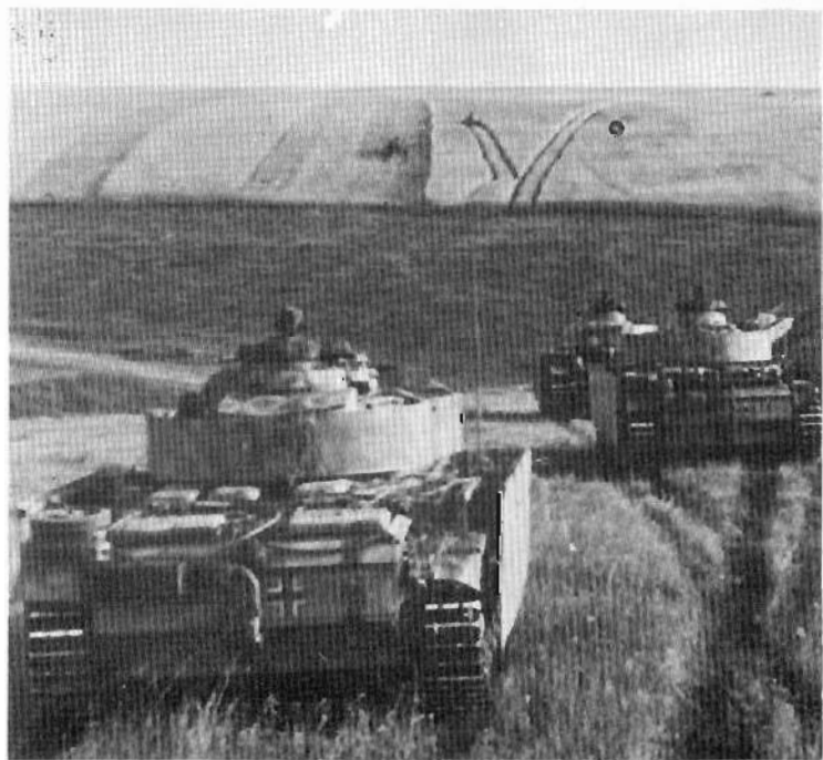
Plates 206-207. Pz Kpfw III Ausf M. Note the modified exhaust valve for deep wading and the absence of both the hull escape hatch and the loader's vision port in the turret side. Right: vehicles equipped with Schürzen (apron armour) on the Russian Front.
