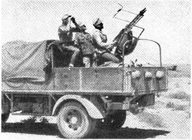
Plate 765. Kfz 4 based on the BMW le gl Einh PKW 4 x 4. Plate 768. The Zwillingssieferts 36 mounted on a medium truck.
