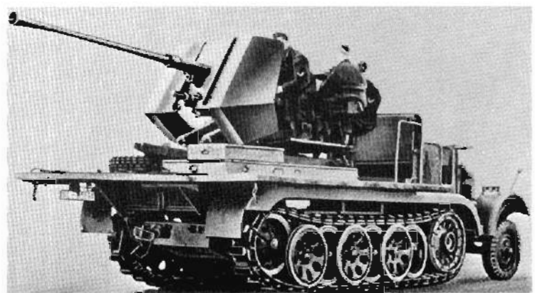
Plates 666-667. 3.7cm FlaK36 auf Fgst Zgkw 5t; right, with gun shield, and lowered sides to permit full traverse of the gun.
