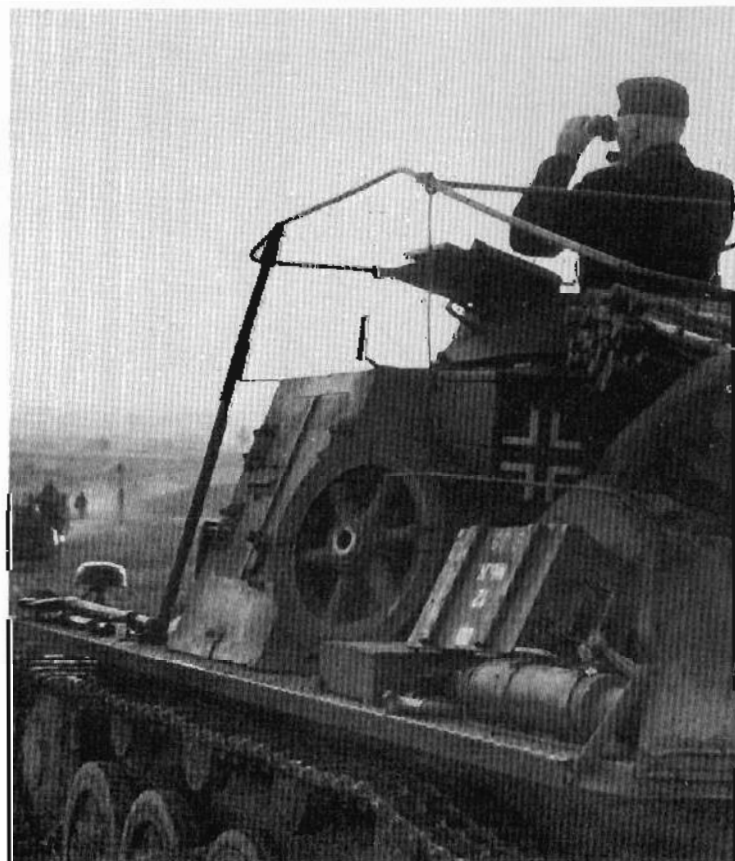
Plate 54. The command vehicle equipped with extra radio equipment and a frame aerial. Plate 55 (opposite page). KI Pz Bef Wg operating in Poland.
