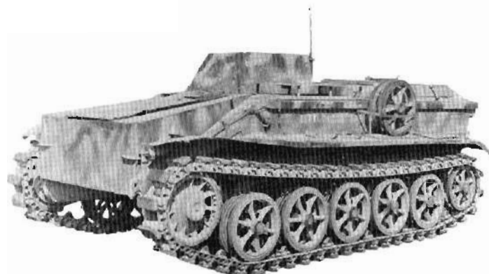
Plate 506. Schwerer Ladungsträger Borgward B III, forerunner of the B IV series. Plates 507-510. Schwerer Ladungsträger Ausf A. In Plate 507, the explosive charge is on the front of the vehicle, and the driver's shields are up. These shields were folded down when the machine was radio-controlled; Plate 509 shows the explosive charge being released. Plate 510, the driver has just the side-shields up.
