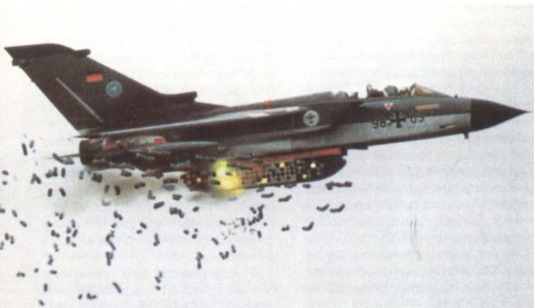
Above: Marineflieger Tornado with MW-1 bomblet dispenser.
