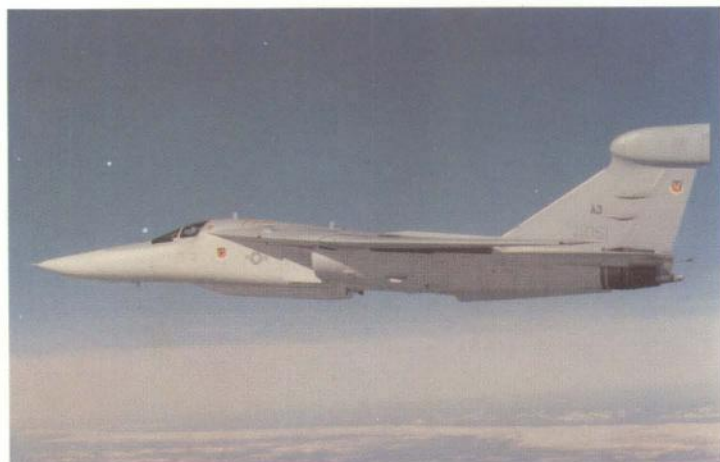
Above: The Electric Fox (EF-111A) is an F-111A rebuilt by Grumman for electronic warfare.
