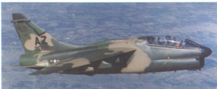
Above: Final production Corsair was the A-7K, a combat-capable two-seater for the US Air National Guard. This particular K went to the 162nd Tactical Fighter Training Group, Arizona ANG.
