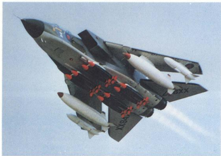
Above: A 1975 picture of the third prototype carrying ECM pods, tanks and eight dummy bombs of low-drag 1,000lb (Mk 83) type.
