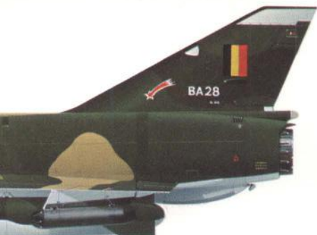
Left: Though amazingly maladjusted to the need, in having very fast takeoff and landing and poor all-weather avionics, the Mirage 5BA, of the FAB (Belgian air force) has long enjoyed some of the best inbuilt ECM of any tactical aircraft in NATO. Loral, the supplier, is likely to equip many F-16s.
