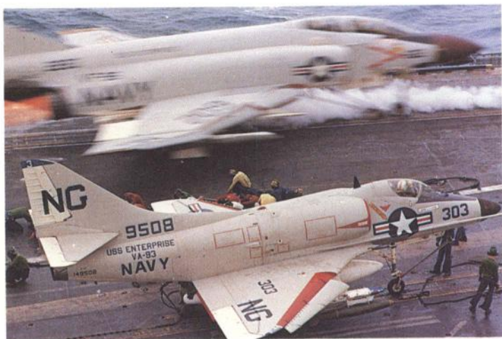
Above: The Skyhawk's tall but narrow landing gear was expected to cause deck stability problems, but did not in use.
