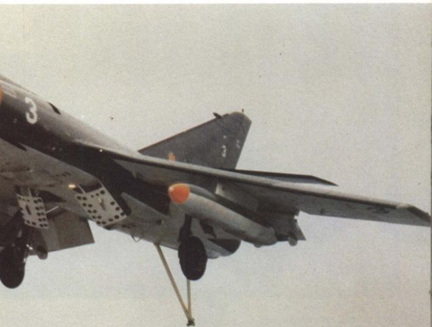
Above: Steam-catapult launch of the eighth Super Etendard, carrying the usual underwing tanks. Note the tailplane angle.
