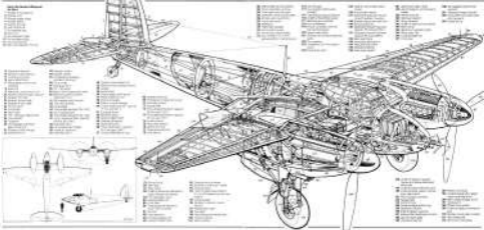
View of the Mosquito's wing structure, showing the wooden framework and engine placement.
